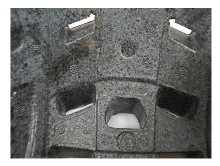
Some helmets held up very well. The molded in the shell helmets have polycarbonate shells to withstand the heat of the molding process. The glued-on or taped-on shells typically have thinner PET or other plastic shells and are more prone to warping in heat. But even some of those held up well.
