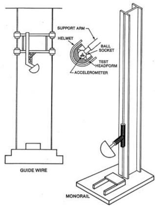
Following the schedule (previous page), drop each helmet on the appropriate anvil. A helmet dropped on the flat anvil has to hit the anvil at a specific velocity, about 20 ft/sec (6.2 m/sec), which typically means that the helmet must drop at least 6 ½ feet (2 m). A helmet dropped on the hemispherical or curbstone anvil has to
